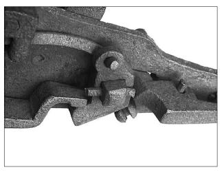
The "push-rod" attached to the tumbler opens the pan-cover as the cock moves forward
