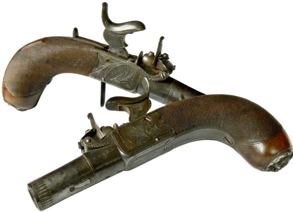
Figures 6-8 - A pair of "top-hat" percussion pistols of fine quality, iron frames signed Sykes, Oxford, c1825, each nipple with sprung cap retainer, finely chequered grips with silver lion-mask butt caps, Birmingham proof marks (courtesy of Scotney Castle, National Trust).
