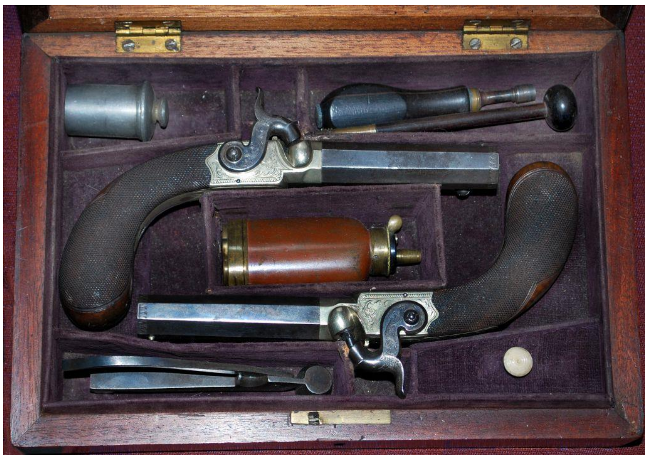
Figures 13 & 14 – A cased pair of percussion overcoat or travelling pistols (courtesy of John Slough of London). These are boxlock, side-hammer pistols, fitted with spring bayonets (on left side of pistol) and cast silver butt caps, complete with a full set of accessories.
