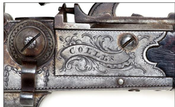
Figures 23 -24 – An over and under double barrelled tap action pistol ( private collection ). This is an early example of the tap-action format. The action, including the tap, is finely engraved and the comb of the cock has a pronounced forward curl. This would suggest that it was made before 1800 despite the use of a folding trigger, which is usually a later feature. The breech is struck with Tower private proof marks. Overall, the pistol is of much better quality than most examples of its type which were made from 1800 onwards, usually in Birmingham.
