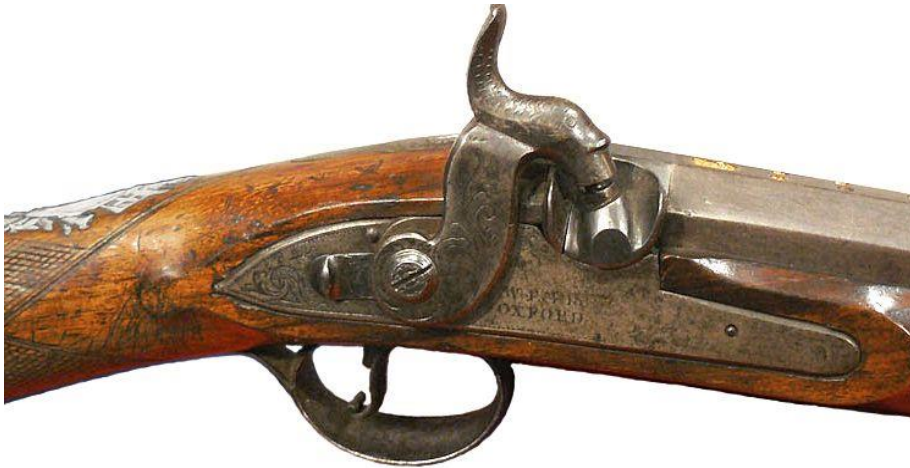
Figures 18-20 A silver mounted sporting gun, with a Spanish barrel by Valero, converted to percussion (pictures courtesy The Lanes Armoury, Brighton ). The lock is fitted with a safety bolt, and is signed "W Emms Oxford". The silver furniture is of particularly high quality. Apart from the Spanish maker's marks, there is a single "V" mark on the barrel.
