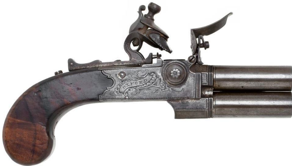
Figures 23 -24 – An over and under double barrelled tap action pistol ( private collection ). This is an early example of the tap-action format. The action, including the tap, is finely engraved and the comb of the cock has a pronounced forward curl. This would suggest that it was made before 1800 despite the use of a folding trigger, which is usually a later feature. The breech is struck with Tower private proof marks. Overall, the pistol is of much better quality than most examples of its type which were made from 1800 onwards, usually in Birmingham.
