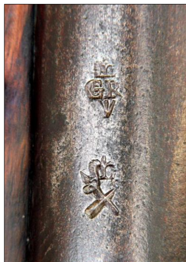
Figure 1 - The Kings Proof mark - consisting of both a proof mark and view mark. Introduced during the reign of Queen Anne in the early 18th century, it was used on all Ordnance made gun barrels
