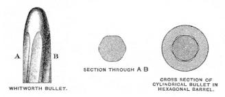
Whitworth's rifling was a radical departure from that used on the current service rifles, being of hexagonal form and shooting a mechanically fitting bullet (see figure above). It should be noted that the polygonal rifling was not an original idea, having been previously considered by that great engineer, Isambard Brunel.
