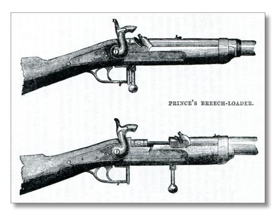
Pictured overleaf is Prince's original patent granted in 1855, it shows the 'bolt handle' positioned off to the side of the rifle's breech in the position we are more accustomed to seeing it. The handle still acts as a locking mechanism for the breech block and the system remains the same as seen in the rifle's built later. The patent also mentions the use of an interrupted screw thread to seal the breech and the possible use of rubber gas seals to prevent venting.
